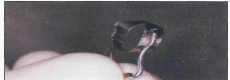
Fig. 6: Second spot welding done for stability.
